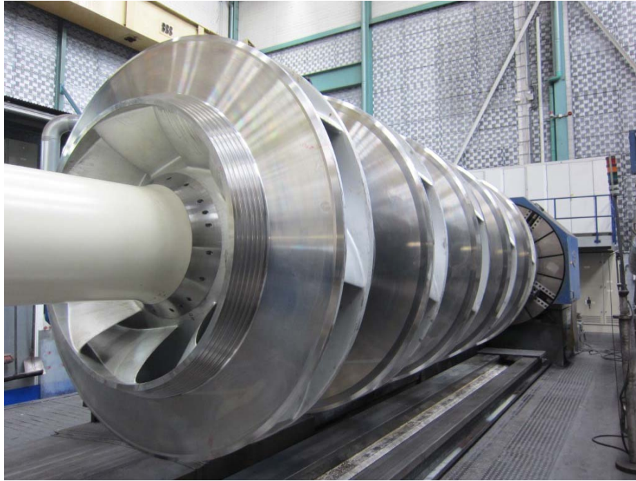
Figure 7: Dimensional Check of the Rotor in Voith Paper's Workshop
